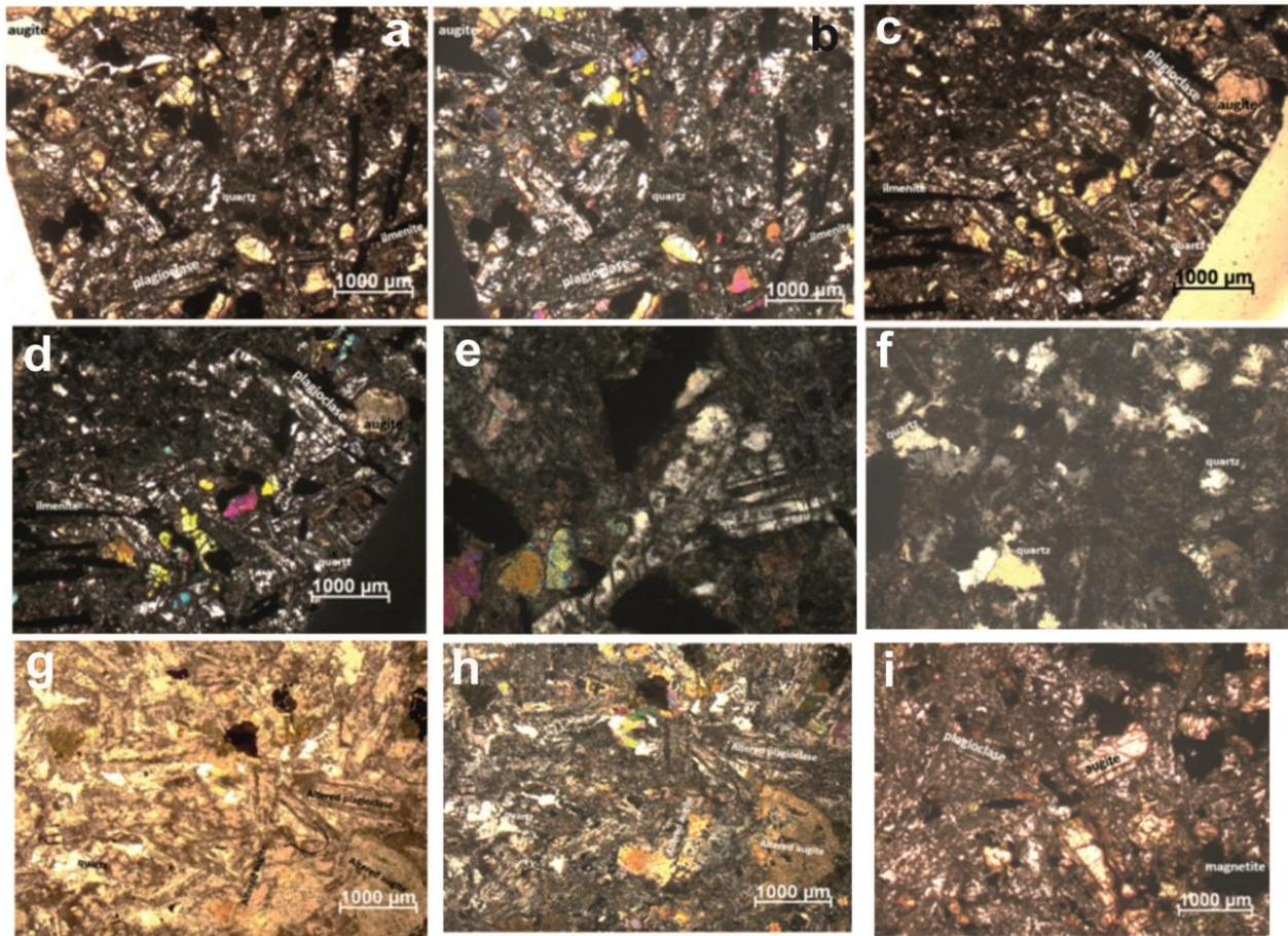
**Fig. 11.** Microstructure of dolerite with quartz, Daouba Kassai: (a–h – sample RU4; i – sample RU7).
