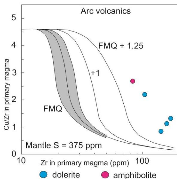
**Fig. 15.** Estimated mantle oxygen fugacities after [14]. Quantitative estimation on mantle redox states beneath arc with varied mantle sulfur contents using Cu/Zr vs. Zr variations for primary arc magmas. The black dashed lines show the mantle melting models with different mantle sulfur contents at  $fO_2 = FMQ$ .
