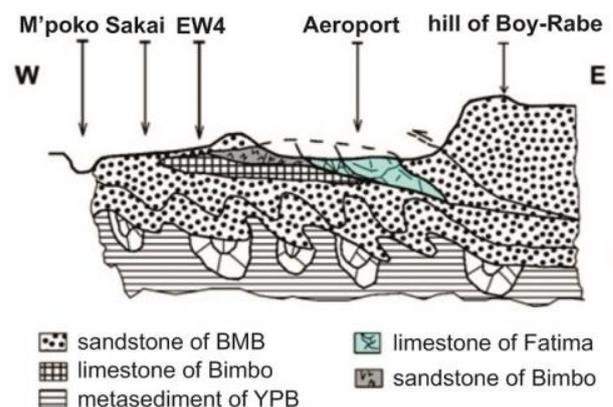
**Fig. 4.** Schematic section illustrating the possible geometry of the geological formations of the Bangui area in the second hypothesis (redrawn after [6]).
