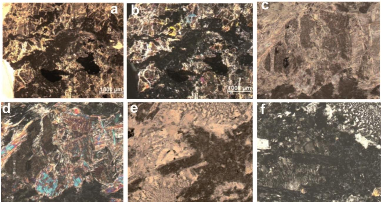
**Fig. 12.** Microstructure of altered dolerite with quartz, Bangui, (RU6).
