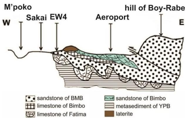
**Fig. 3.** Schematic section illustrating the hypothetical geometry of the geological formations of the Bangui sector in the first hypothesis (redrawn after [6]).
