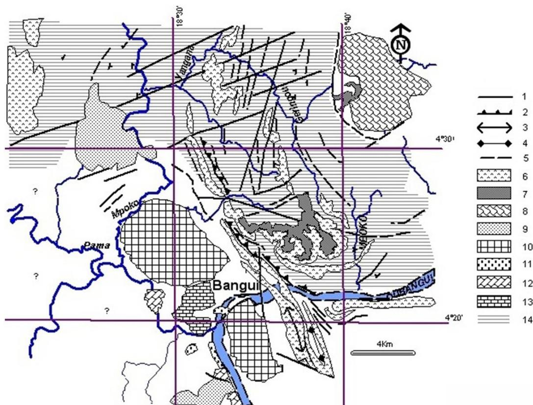
**Fig. 2.** Location of major geological units (after [1] reproduced by [6]). Legends: (1) – direction of schistosity; (2) – overlap; (3) – anticline axis; (4) – syncline axis; (5) – fractures and faults; (6) – quartzite; (7) – cuirasse; (8) – amphibolite and micaschist; (9) – quartzite, sandstone; (10) – karstic morphology; (11) – conglomerate; (12) – chert and limestone; (13) – limestone recognised by sounding; (14) – chlorite and sericite schists (YPB).
