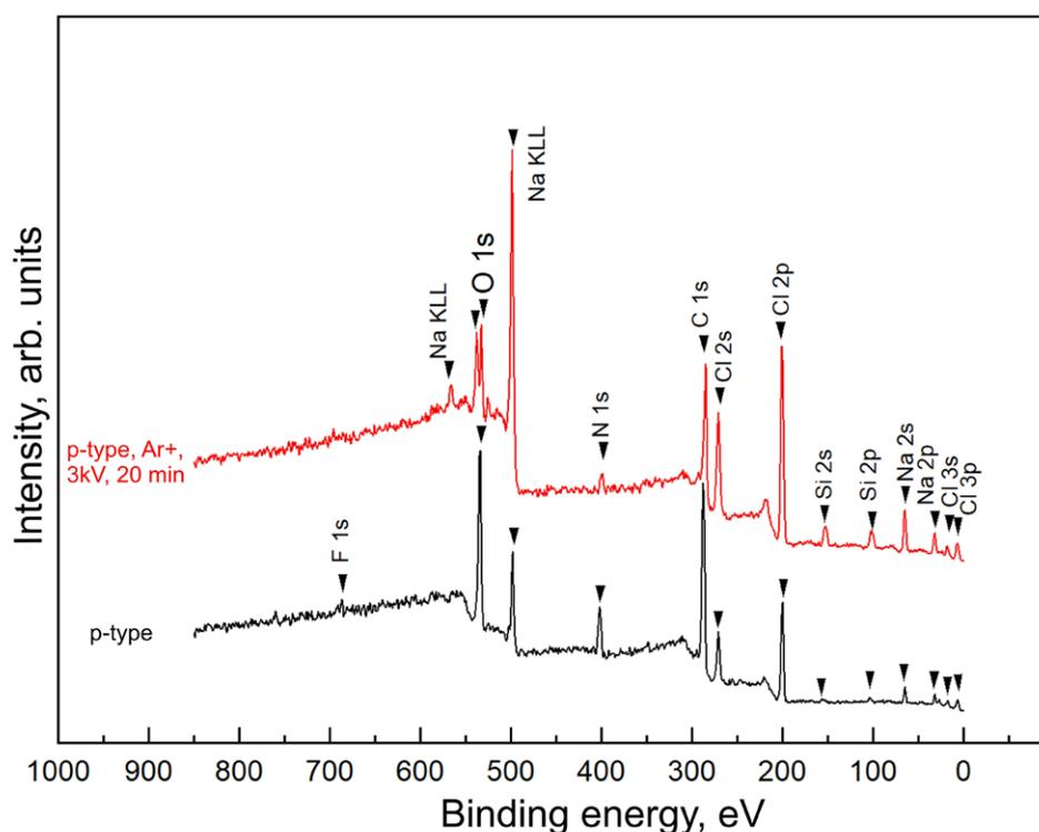
**Fig. 2.** XPS survey spectra of a silicon wires sample formed on a *p*-type substrate before (black) and after (red) ion beam etching ( $\text{Ar}^+$  3 kV 20 min). The characteristic elements that make up the studied sample surface are noted
