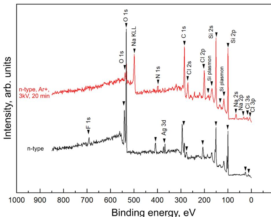
**Fig. 3.** XPS survey spectra of a silicon wires sample formed on a *p*-type substrate before (black) and after (red) ion beam etching (Ar+ 3 kV 20 min). The characteristic elements that make up the studied sample surface are noted
