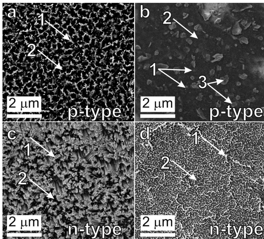
**Fig. 1.** Scanning electron microscopy of the initial samples of silicon wires array surfaces formed from *p*-type (a) and *n*-type (c) substrates, as well as after layering of the Dps protein molecular culture (b) and (e), respectively. 1 – tops of wires (walls of pores), 2 – pores between wires, 3 – NaCl salt particles after drying
