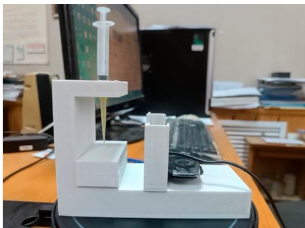
**Fig. 2.** Installation for measuring contact angles
