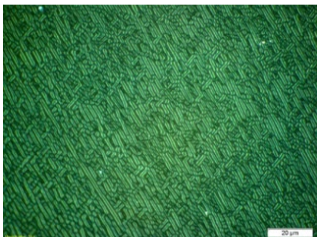
Fig. 6. Micrograph of lithium niobate sample after proton exchange (175 °C, 6 h) and annealing (370 °C, 2 h)
