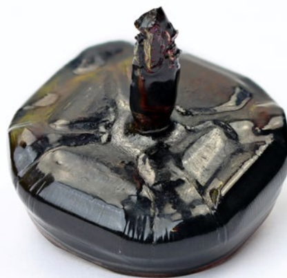
Fig. 4. Photograph of a crystal \text{NaBa}_{12}(\text{BO}_3)_7\text{F}_4 ( P4_2bc ), 28 \times 28 \times 11 mm, grown in the system Na, Ba, B // O, F from a composition of 38 mol % BaO, 13 mol % \text{Na}_2\text{O} , 13 mol % \text{Ba}_2\text{O}_3 , 36 mol % \text{BaF}_2
