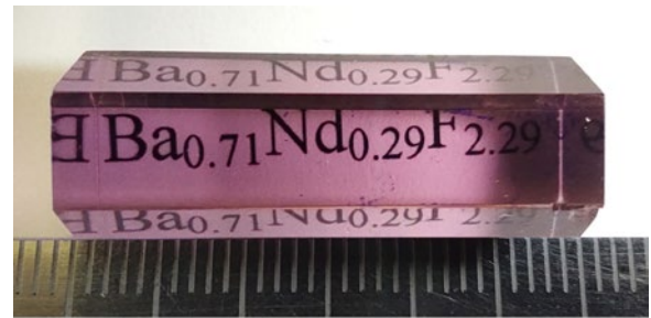
Fig. 9. Single crystal of Ba_{0.71}Nd_{0.29}F_{2.29} – optical filter for a wavelength of 2.5 \mu m . The faceting is artificial. Grown by T. Turkina [54]. Photographed January 22, 2024
