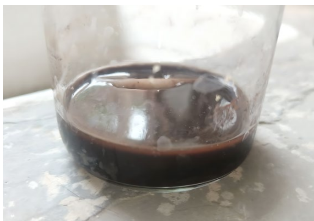
Fig. 4. Graphene oxide obtained from graphitic carbon
