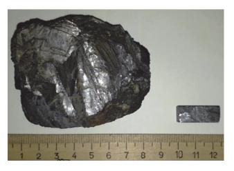
**Fig. 1.** Photo of a galena monolith with a piece cut off for a sample
