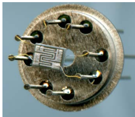
Fig. 1. The test structure used for the analysis of the electrophysical and gas sensitivity properties of the PdO films
