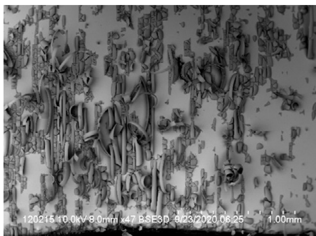
Fig. 6. Micrograph of Mn_5Ge_3 surface after 10 minutes anodic polarization at E = + 0.6V in a 0.5 M Na_2SO_4 solution
