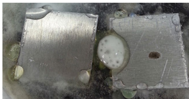
Fig. 9. The formation of hydrogen produced during the interaction of exudate with the D16T alloy at the sites of its contact with the lawn of micromycete mycelium.
