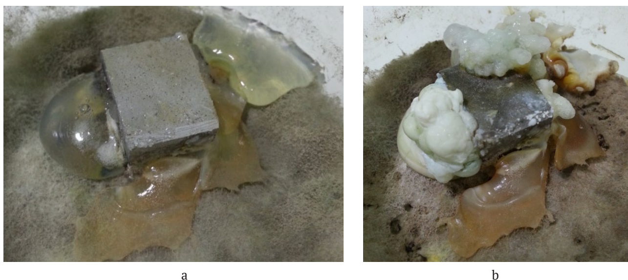
Fig. 10. Biocorrosion products of the alloy: gel and jelly at the sites of exudate formation (a); crystalline corrosion products (b)
