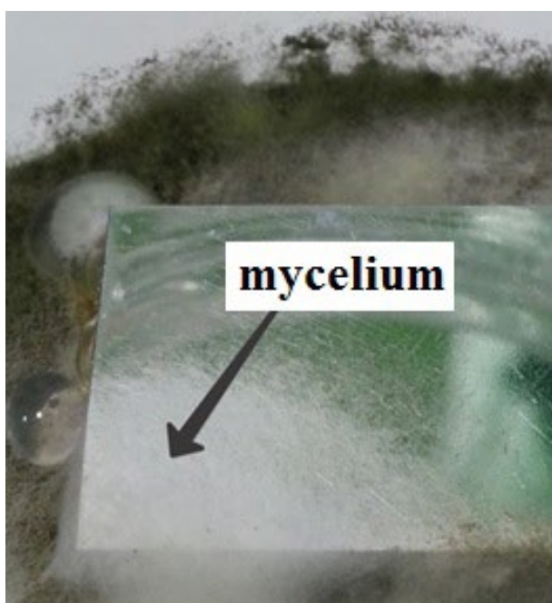
Fig. 6. Adhesion of mycelium of micromycetes on the surface of the samples and their gradual overgrowth (shown by arrows)
