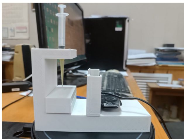
Fig. 3. The original setup for measurement of the contact angle, printed on a Hercules Original 3D printer
